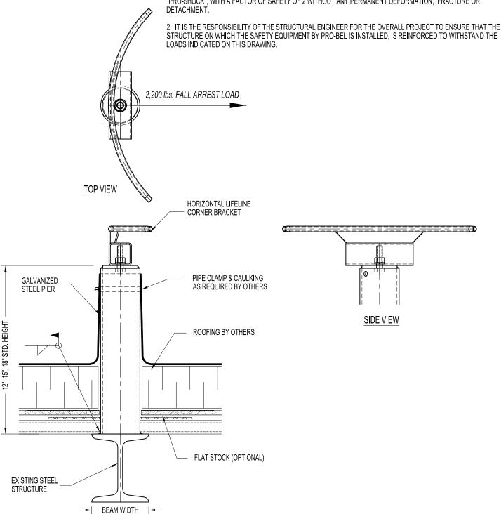
HLL-75C1-0000: WELD TO STRUCTURE HLL CORNER ANCHOR
