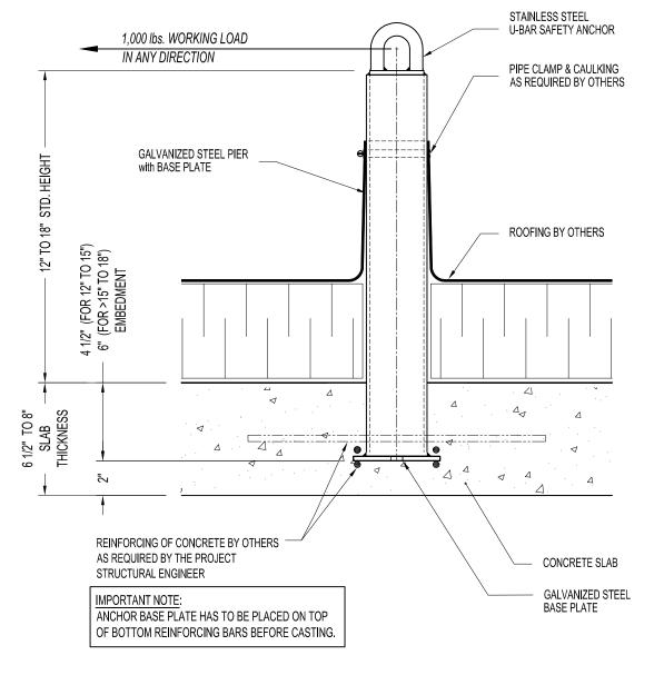
PBE74EBD: FULLY EMBEDDED IN CONCRETE SLAB ROOF ANCHOR
