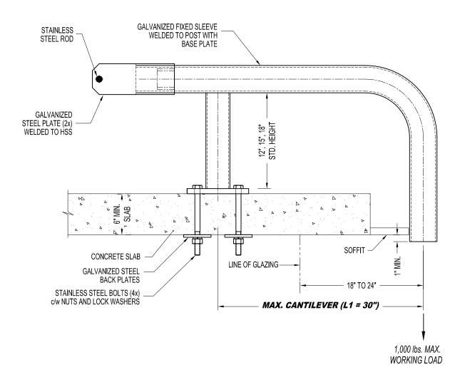
A-RSC14111: BOLT THROUGH CONCRETE - CURVED RIGGING SLEEVE (4" O.D. FIXED SLEEVE)
