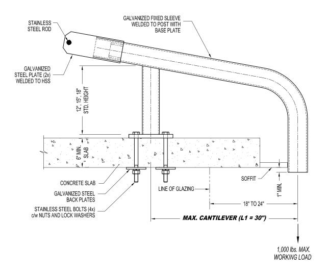
A-RSC04111: BOLT THROUGH CONCRETE - CURVED RIGGING SLEEVE (4" O.D. FIXED SLEEVE)
