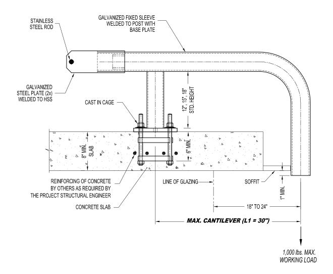
A-RSC14131: CAST IN CAGE - CURVED RIGGING SLEEVE (4" O.D. FIXED SLEEVE)
