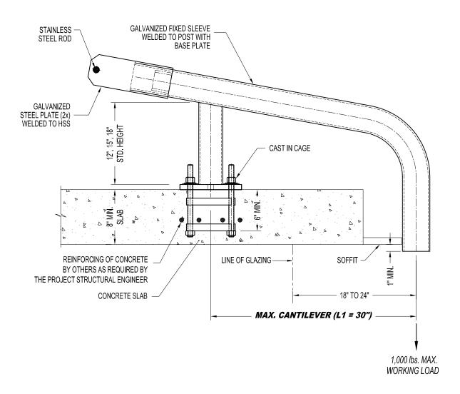
A-RSC04131: CAST IN CAGE - CURVED RIGGING SLEEVE (4" O.D. FIXED SLEEVE)
