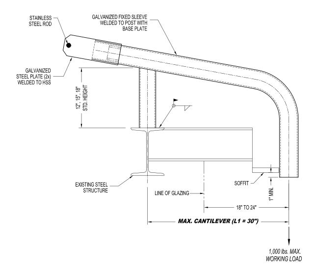
A-RSC04151: WELD TO STEEL - CURVED RIGGING SLEEVE (4" O.D. FIXED SLEEVE)
