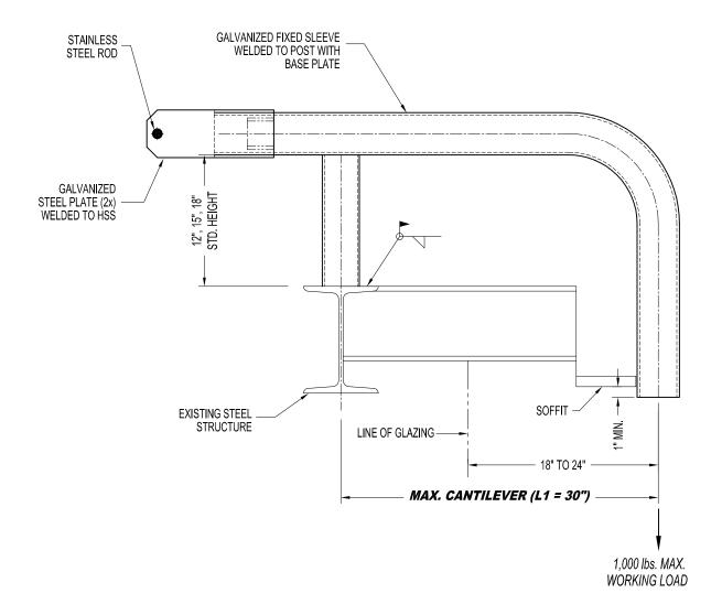
A-RSC14151: WELD TO STEEL - CURVED RIGGING SLEEVE (4" O.D. FIXED SLEEVE)
