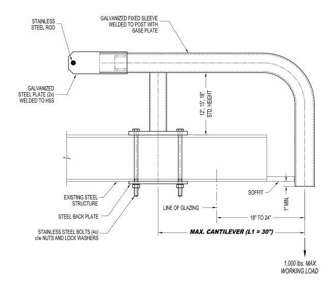
A-RSC14141: WRAP AROUND STEEL - CURVED RIGGING SLEEVE (4" O.D. FIXED SLEEVE)
