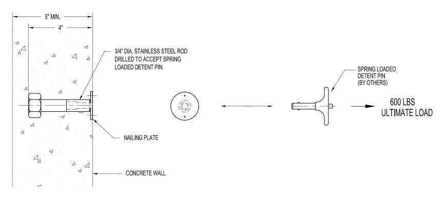
A-STB-RDN1312-04: CAST INTO CONCRETE (FLUSH MOUNTED) STABILIZATION TO SUIT SPRING LOADED DETENT PIN
