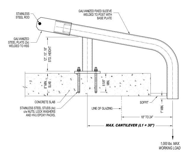
A-RSC04171: ADHESIVE - CURVED RIGGING SLEEVE (4" O.D. FIXED SLEEVE)
