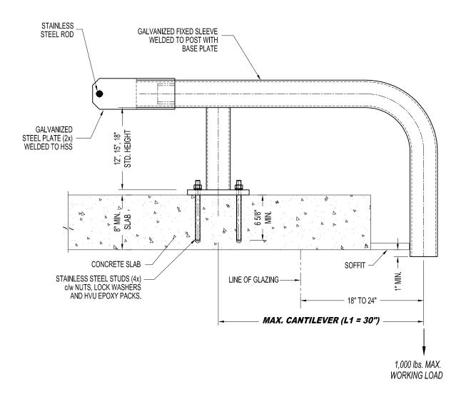
A-RSC14171: ADHESIVE - CURVED RIGGING SLEEVE (4" O.D. FIXED SLEEVE)
